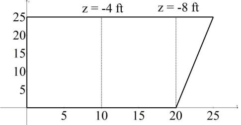
The bottom of the pool is a plane with depths as indicated (the pool gets deeper in a linear way from left-to-right)
